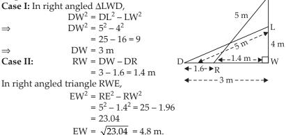
:. The distance by which the ladder shifted upward = EL = 4.8 m - 4 m = 0.8 m
