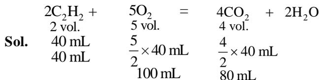
So, for complete combustion of 40 mL of acetylene, 100 mL of oxygen are required and 80 mL of carbon dioxide are formed.
