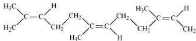
Because of this cis-configuration, intermolecular interactions between the various strands of isoprene are quite weak. As a result, various strands in natural rubber are arranged randomly. Hence, it shows elasticity.
