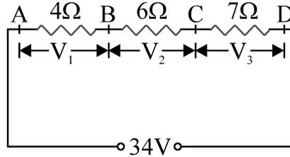
**Sol.** The current through the circuit =  $\frac{34V}{(4 + 6 + 7)\text{ohm}} = 2A$
