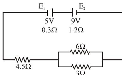
74. Calculate the current shown by the ammeter in the circuit diagram given below in figure :
