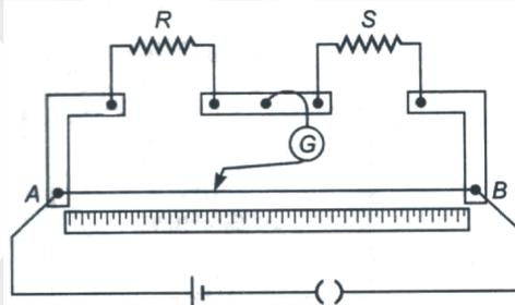
48. In a meter bridge, the null point is found at a distance of  $l_1$  cm from A. If a resistance of  $X$  is connected in parallel with  $S$ , the null point occurs at a distance  $l_2$  cm from A. Obtain the formula for  $X$  in terms of  $l_1$ ,  $l_2$  and  $S$ . [Delhi 2010]
