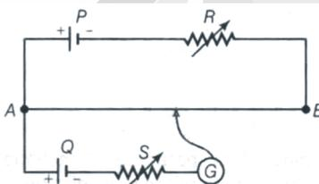
In the potentiometer circuit shown in the figure, the balance point is at X. State, giving reason, how the balance point is shifted when (i) resistance R is increased (ii) resistance S is increased, keeping R constant? [Comp.2013]
