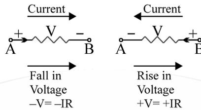
It is clear that the sign of voltage drop across a resistor depends on the direction of current through that resistor but is independent of the polarity of any other source of e.m.f. in the circuit under consideration.
