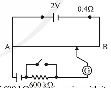
To ensure very low currents drawn from the standard cell, a very high resistance of  $600\text{ k}\Omega$  is put in series with it, which is shorted close to the balance point. The standard cell is then replaced by a cell of unknown emf  $\epsilon$  and the balance point found similarly, turns out to be at 82.3 cm length of the wire.
