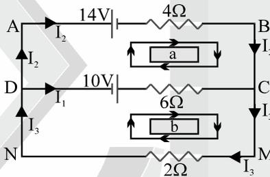
**Sol.** Junction rule at C yields  $I_1 + I_2 - I_3 = 0$  i.e.,  $I_1 + I_2 = I_3$  ....(1)
