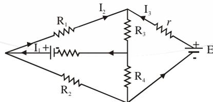
73. Two cells  $E_1$  and  $E_2$  in the given circuit diagram have an emf of 5V and 9V and internal resistance of  $0.3\Omega$  and  $1.2\Omega$  respectively. Calculate the value of current flowing through the resistance of  $3\Omega$ .
