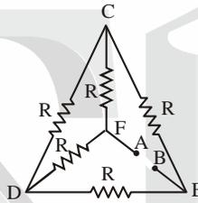
(ii) Also calculate the current through CD and ACB, if a 10 V d.c. source is connected between A and B and the value of R is assumed as  $2\Omega$ .
