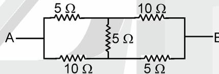
Sol. It is wheat stone bridge but not balanced. No series parallel connections. But similar values on input side and output. Here we see that even after using symmetry the circuit does not reduce to series parallel combination as in previous examples.
