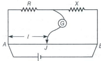
46. In a meter bridge, the null point is found at a distance of 40 cm from A. If a resistance of  $12\Omega$  is connected in parallel with  $S$ , the null point occurs at 50.0 cm from A. Determine the values of  $R$  and  $S$ . [HOTS; Delhi 2010]
