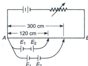
Find (i)  $E_1/E_2$  and (ii) position of null point for the cell  $E_1$ . How is the sensitivity of a potentiometer increased?
