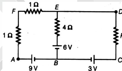
36. Calculate the value of the resistance R in the circuit shown in the figure so that the current in the circuit is 0.2 A. What would be the potential difference between points A and B? [All India 2012]
