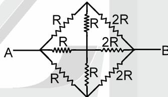
**Sol.** In this case the circuit has symmetry in the two branches AC and AD at the input
