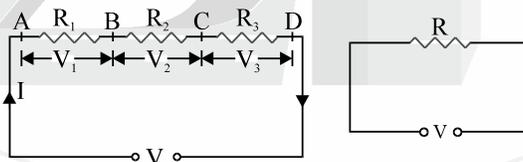
$$\therefore V = V_1 + V_2 + V_3 = IR_1 + IR_2 + IR_3 \quad (\text{Ohm's Law})$$
