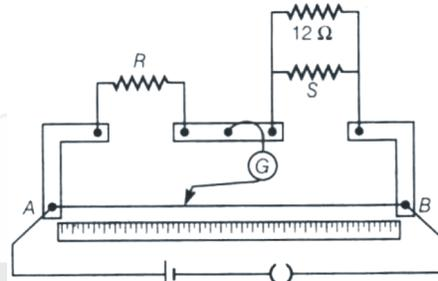
47. In a meter bridge, the null point is found at a distance of 60 cm from A. If a resistance of  $5\Omega$  is connected in series with  $S$ , the null point occurs at 50.0 cm from A. Determine the values of  $R$  and  $S$ . [Delhi 2010]
