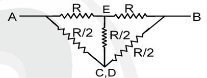
2. Find the equivalent Resistance between A and B
