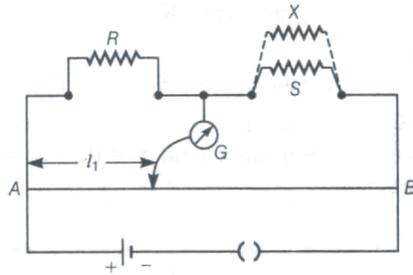
50. Draw a circuit showing a Wheatstone bridge. Use Kirchhoff's rule to obtain the balance condition in terms of the values of the four resistors for the galvanometer to give null deflection. **[Delhi 2008C]**
