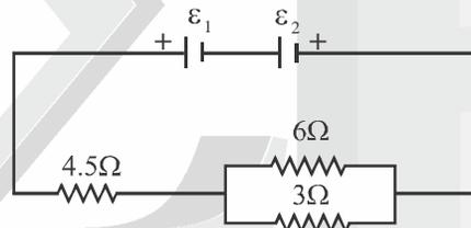
Calculate the value of current flowing through the resistance of  $3\Omega$ .
