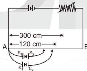
54. A potentiometer wire of length 1 m has a resistance of  $10\ \Omega$ . It is connected to a 6 V battery in series with a resistance of  $5\ \Omega$ . Determine the emf of the primary cell which gives a balance point at 40. **[2014]**
