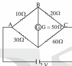
What is the current flowing in the arm BD of this circuit? State the two laws used to find the current in different branches of this circuit?
