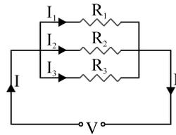
$$I = I_1 + I_2 + I_3 = \frac{V}{R_1} + \frac{V}{R_2} + \frac{V}{R_3}$$
